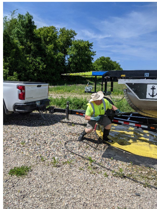
Figure 7. A level 2 inspector decontaminating a barge with high pressure
