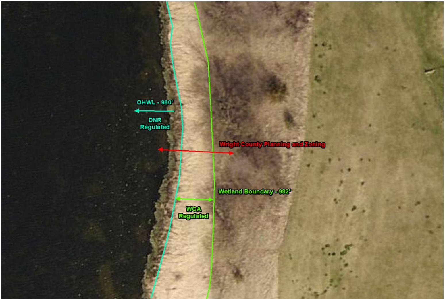
The above figure shows an example of where jurisdictions may exist for a project. The Ordinary High-Water Level (OHWL) designates the elevation in which a permit may be required through the DNR. The Wetland Boundary designates the actual extent of wetlands along the shoreline subject to MN Wetland Conservation Act rules, and the red line designates those projects within the OHWL, Wetland Boundary, and above may require a permit through Wright County Planning and Zoning.
