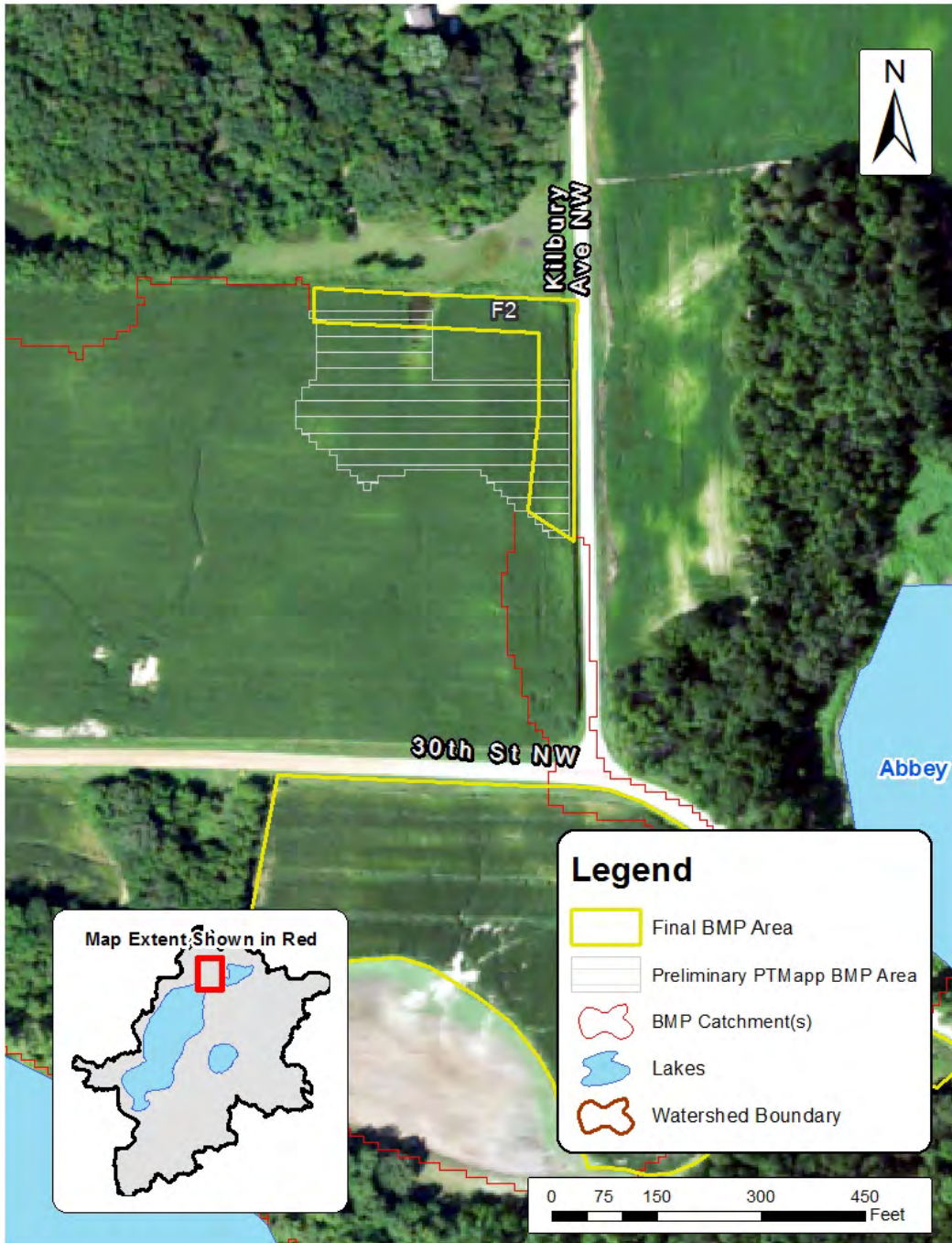
Figure 12. Field scale map of BMP F2, a filter strip. The white shaded area is what PTMapp originally delineated and the yellow outline is Wright SWCD staff estimate
