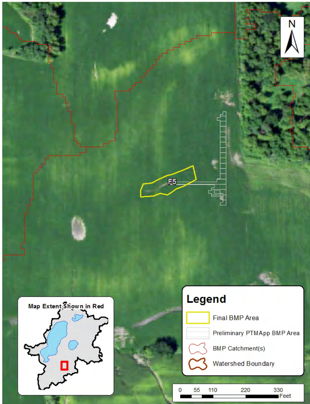
Figure 18. Field scale map of BMP F4, a grassed waterway. The white shaded area is what PTMAApp originally delineated and the yellow outline is Wright SWCD staff estimate
