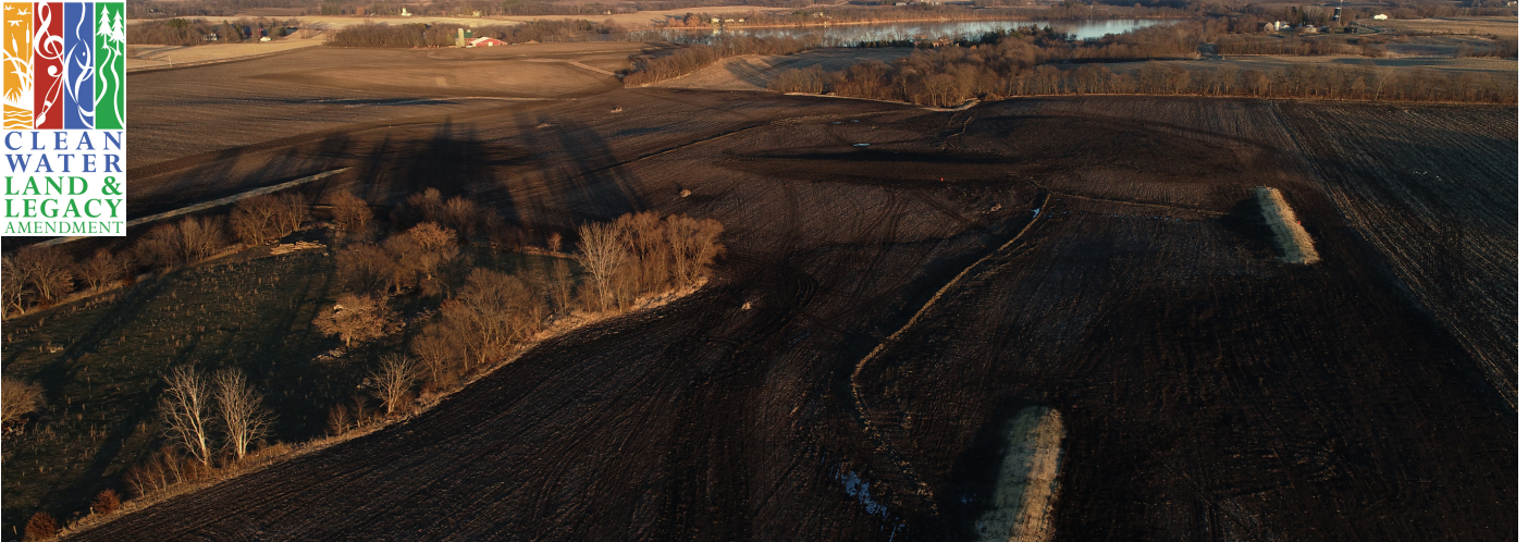
Seven water and sediment control basins completed in Albion Township. This will stop eroded sediment from reaching Camp Lake and help to improve the producer's yield.
