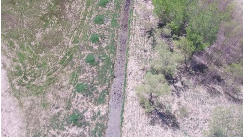
Figure 20. Vegetation Growth in Open Ditch (Cattails) Section 5 Victor Township on Tuey Lateral
